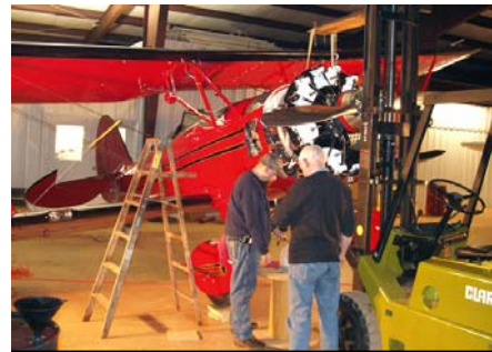
Unusable Fuel Test – right slip
