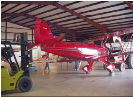
Unusable Fuel Test – left slip
