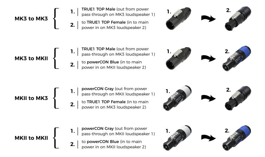
\*The combined current draw of all speakers in a chain must not exceed the current rating of the outlet or any individual connector. Connect subwoofers first in the chain and then chain from subs to tops.
