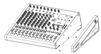
3. Using only the new screws supplied, secure the rack ear brackets to each side of the mixer as shown below. Tighten the screws securely using the Phillips screwdriver. Be sure not to overtighten. As seen in the illustration below, they require six screws (three on each side).
