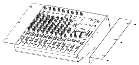
4. Offer up the mixer to the rack and secure it in place with four rack screws (not supplied). Remember to leave enough room at the top to attach the AC power cord and any other connections needed.
