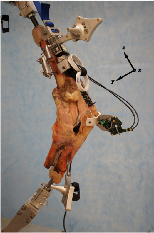
Fig. 2. Placement of the active infrared surgical navigation trackers and the tibiofemoral coordinate system.
