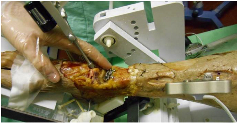
Fig. 5. Cadaver specimen positioned in the testing rig during data acquisition; the ankle is replaced with one of the prototypes.
