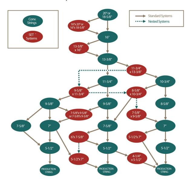
Depending on required parameters, not all SET System liners may be installed as shown. Each installation must take into consideration hole conditions, base casing weight, expansion ratio, and required clearance. Nested systems are SET Systems installed inside of each other and require specific expansion ratios.
