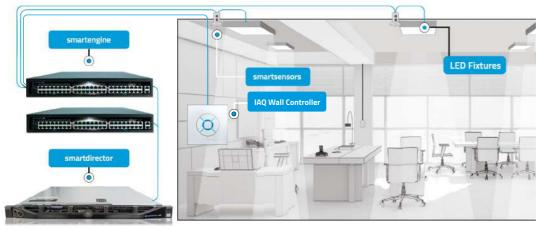
The smartdirector provides a browser based user interface for all of the smartengine devices, stores smartsensor data and provides web services and BACnet/IP APIs.
