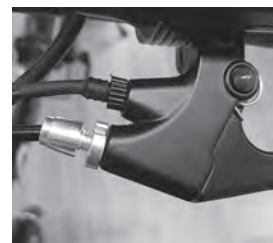
Applying the brakes activates the brake sensor which cuts the power to the motor.
