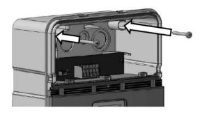
Use the *strain relief* (*small/large*) for the installation type "from the bottom" or "from the top" of the connection cable.
