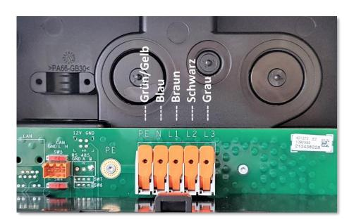
Prepare the connection cable by shortening the individual wires to the correct length and insulate the individual wires with the stripping pliers. The stripping length of the individual wires is 11-13 mm.
