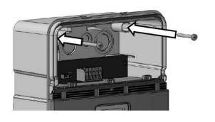
Use the *strain relief* (*small/large*) for the installation type "from the bottom" or "from the top" of the connection cable.
