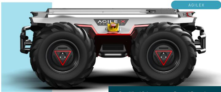
This chassis can be installed with different upper load and navigation system for inspection, transportation, teaching and other scenarios.
