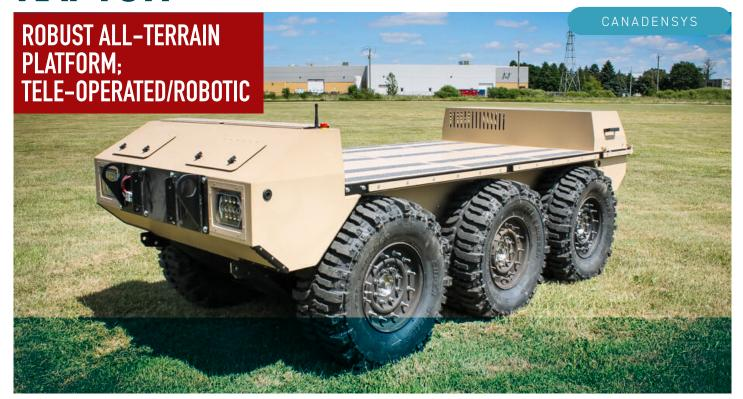
RAPTOR is a multi-purpose mobility platform designed to travel over extreme terrain in any weather conditions. Target environments include jungle, desert, arctic snow, tundra, swamp, and water conditions. A powerful
