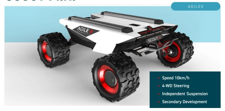
SCOUT MINI is a member of the SCOUT mobile robot family and inherits the advantages of SCOUT -4WD, independent suspension, and in-place self-rotation.
