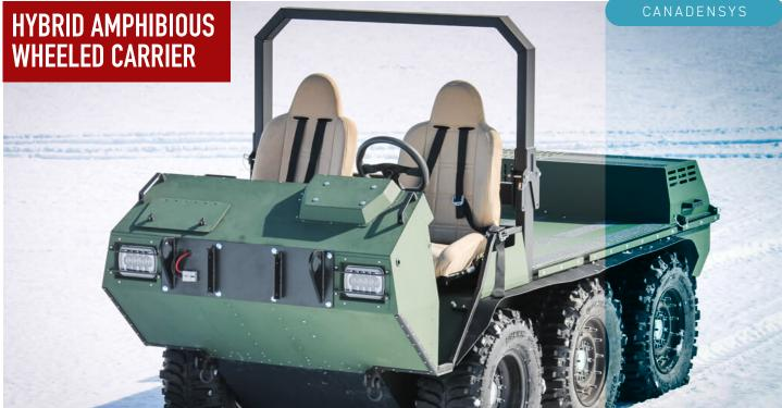
HAWC is a multi-purpose mobility platform for movement of personnel and/or equipment over extreme terrain environments in any weather conditions. Target environments include jungle, desert, arctic snow, tundra, swamp, and water conditions. A powerful integrated diesel generator (optional) provides continuous running capability, while a 96V battery pack allows the vehicle to be operated in an emissions-free, near-silent mode.
