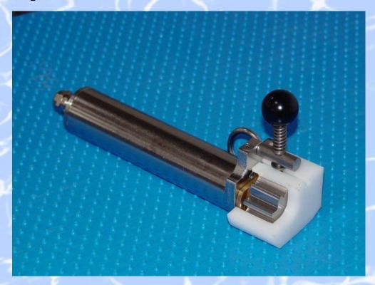
Tiny and smart hand held pinbone remover developed on the same principles as the well-known EASY-MATIC pinbone removers.
