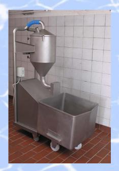
The vacuum system removes the bones and the water from the filets and leaves the filets clean and dry.
