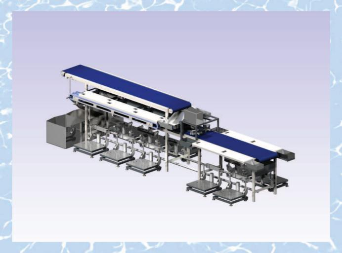
Trimming line with pinbone remover is a compact unit taking care of trimming and pinboning in one process. Trimming line is constructed so the operator don't have to lift the fillets during the process.
