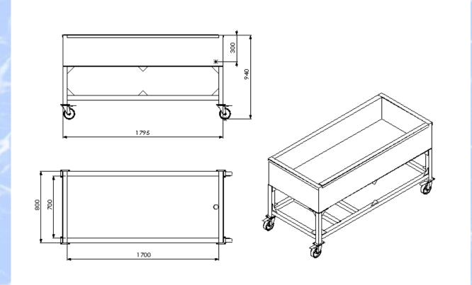
With compressor built in under the vessel. The freezer is isolated in the bottom and sides.
