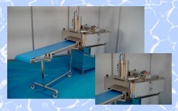
KSL slicer has a capacity up to 250 slices pr. Minute of frozen loins, which have a temperature between -12 to -16 degrees.
