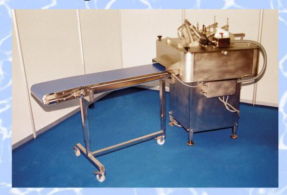
KSL Slicing Machine has a capacity up to 250 slices per minute of frozen fillets at a temperature of -12 to -16 degree Celsius.
