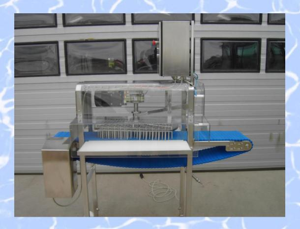
FC 100 is a fish turner, which can turn the fillets in a processing line from tail-end first to head-first or opposite, without using manpower, and therefore is it possible to save an operator between pin bone remover and a possible skinning machine, where the tail-end first is needed.
