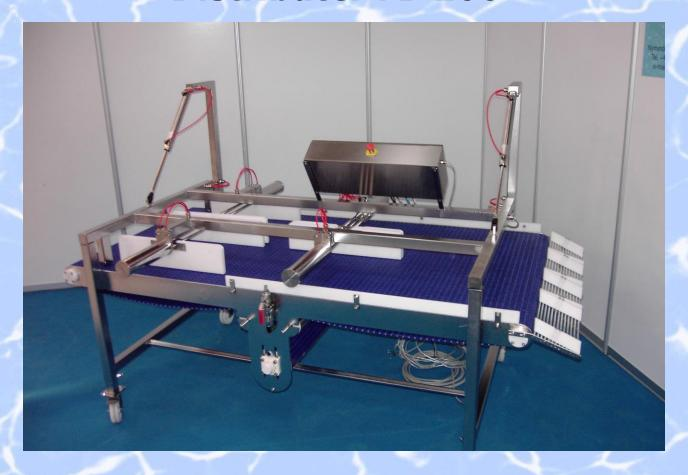
FB 200 Fish Distributor distributes the filets from Baader 988 where the filets come out in 2 lanes into 4 lanes in the pinbone-remover EM204.
