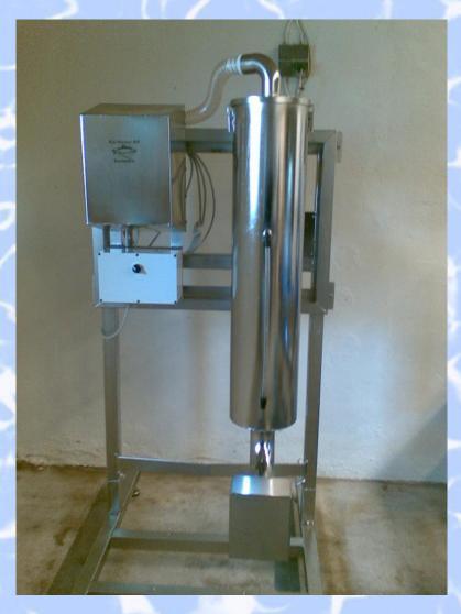
The vacuum system removes the bones and the water from the filets and leaves the filets clean and dry.
