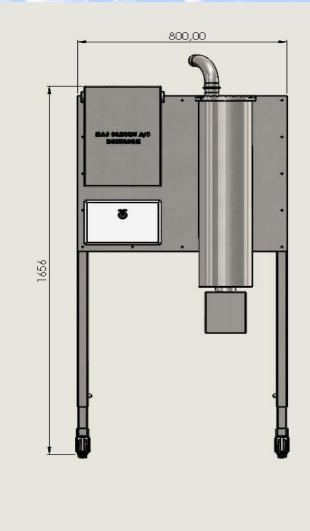
Tank removeable for cleaning.
