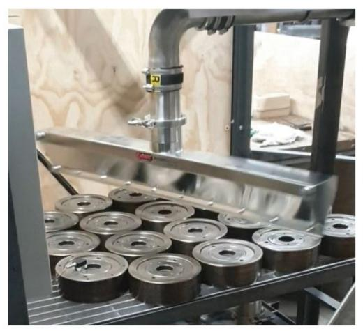
After the regulators are run through this process, they must be thoroughly dried, because any moisture left in the crifices after the regulators are assembled could lead to false gas flow rate readings. Further, the drying mechanism has to be sufficiently gentle to remove the moisture without damaging the regulators, as any surface abrasion on the gasket areas of the castings could produce failures during the pressure check.
