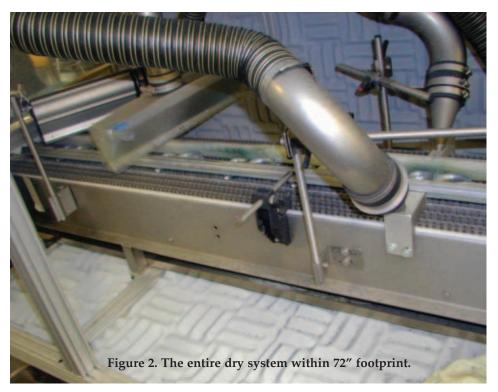
Although LaRoux says he has yet to run tests to determine the exact amount of savings, he estimates the energy cost is much lower since moving away from a compressed air-based drying process. In fact, according to Sonic Air, its air-knife dryers can provide as much as 14-times the energy savings as a compressed air system.
