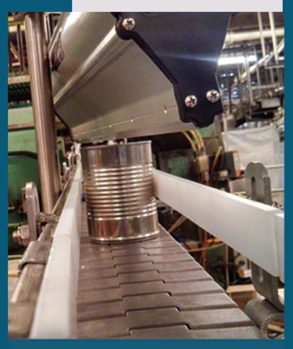
Damp cans are liable to cause all manner of pack failures as well as make printing difficult, so drying is a necessary process in the filling plant.
