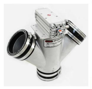
The automated Sonic Y-Verter flow control valve mounts on the outlet of a blower powered air knife system and responds to PLC signals much like a VFD.
