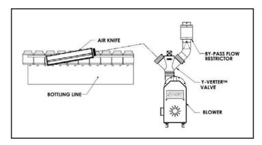
Valves for air knife velocity control can instantly reduce or shut off flow to the production line. They're nearly as efficient as VFDs under most operating conditions. make for a strong justification for the air control valve option.
