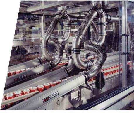
Engineered air-knife systems are often used on high-speed beverage conveyors to remove moisture prior to labeling or ink-jet coding.
