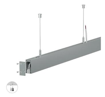
High-quality 6063 thin-wall aluminum, light-weight design featuring hidden cables and suspended by cables from the ceiling. The raceway space is enough to conceal seamless connectors with bottom feed and the general male/female connectors. It is superb for the facade where tidiness is required and the scenarios that lack of space for wiring.
