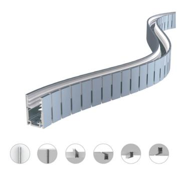
It is an expanded design of the flexible aluminum profile, and caters for the continuously streamlined aesthetics of curve shape. The secondary precision cutting process, not only maintains the advantage of clamping force, but also enables the two-way horizontal bending directions with super shape memory.
