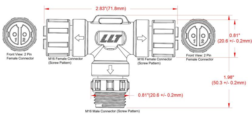
Internal parallel connection, 2 Pin, 15A, IP67.
