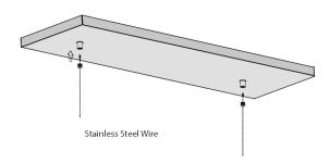
Thread the stainless steel wire through the male cable coupler. Then screw the male cable coupler to the female cable coupler attachment piece.
