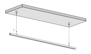
Thread the stainless steel wire through the Cable Gripper Nut and Cable Gripper.
