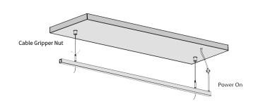
Adjust the length of the stainless steel wires to the desired height and tighten the Cable Gripper Nut. After testing the fixture and confirming the desired position, cut or roll up the excess stainless steel wires.
