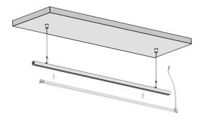
Insert the fixture into the aluminum channel as instructed in the handling guide.
