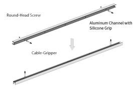
Screw the Hex Bolt to the Cable Gripper. Insert the Round-head Screw into the aluminum channel and through the mounting holes. Screw together the Roundhead Screw and Cable Gripper/ Hex Bolt.
