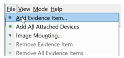
3. Select "image file" as the source evidence type. Ensure both the E01 and E02 files are located in a single folder. Point to the E01 file within the folder. Once the correct location is pointed to in the source path click "finish."
