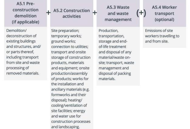
Figure 12: Sub-modules of module A5
