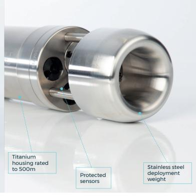
With an operational battery life of up to 5 days and the convenience of charging via USB, SWiFT is intended for coastal, harbour and inland hydrographic surveyuse and offers the highest quality sound velocity profiles in a compact, robust and portable package. Optionally, the supplied deployment weight is available to bolt onto the sensor protection cage to help get the SWiFT to depth in fast flowing currents.
