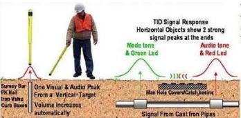
To start search turn sensitivity control up aprox 1/2. Hold tip close to ground & move forward swinging detector left and right. To pinpoint a target hold detector vertically over target object.
