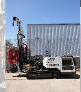
The Klemm 708 is a multi-purpose drill rig for all drilling systems. A series of options is available to provide the optimum rig configuration for a particular drilling process:
