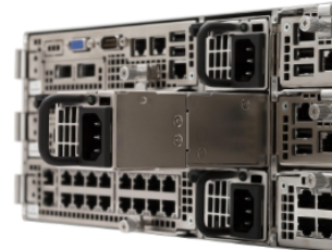
RES Server Dual Redundant Power
