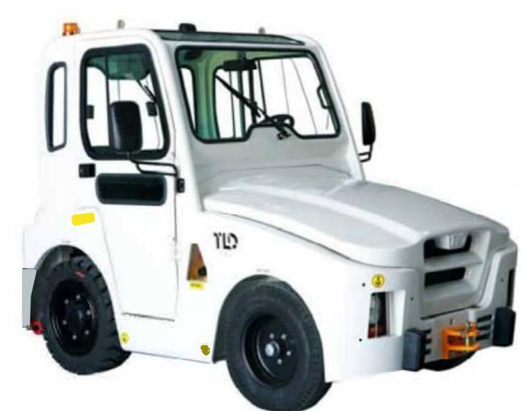
The JST Series towing tractors, available with a maximum draw bar pull ranging from 2,000 daN (4,400 lbs) up to 2,800 daN (6,160 lbs), are designed to tow baggage carts, towable GSE and cargo trailers. JST tractors may be used for exceptional push back operation on small size aircraft, under certain conditions. Please contact manufacturer for details. This unit features a heavy duty frame made of arc-welded steel plate with rear heavy cast iron body to achieve long operating life.
