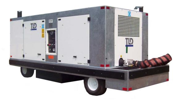
The ASU-600-150 are truck or trailer mounted continuous flow jet engine starting units producing up to 150 PPM and up to 40 psig start air pressure.
