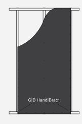
7mm Structural Ply™ fixed with 50 x 2.8mm flat head nails at 150mm centres around perimeter at no less than 7mm from sheet edge. 300mm centres to intermediate studs
