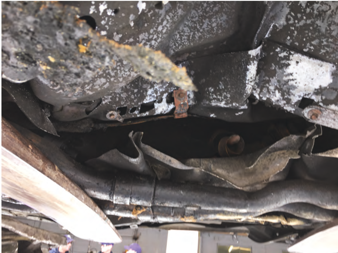
Photo of Lincoln transmission pan resting on exhaust pipes.
