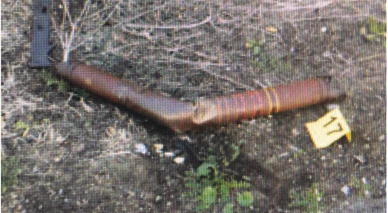
The front drive shaft tore off the transfer case:
