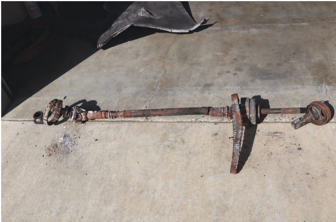
The front drive shaft tore off the transfer case:
