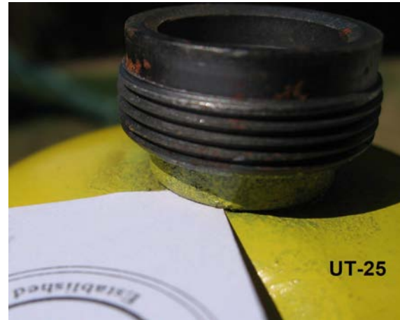
Poorly brazed joint as found on the shelf at Home Depot.
