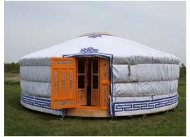
Diameter: 25 to 26 feet (8m) Wall height: 5 1/2 feet(1.7m) Height in center: 9 feet (2.8m)
