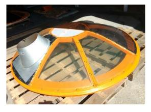
Toono finish 1/2: The front half of the toono (dome) is covered and sealed with acrylic and can be fitted with a chimney flashing for stove pipe passage. The back half of the toono is open and can be covered with mosquito netting and secured with Velcro. In case of rain or cold weather, the back half is covered with the insulated urgh (top flap), which is included with the purchase of your yurt. You can watch a video here:
