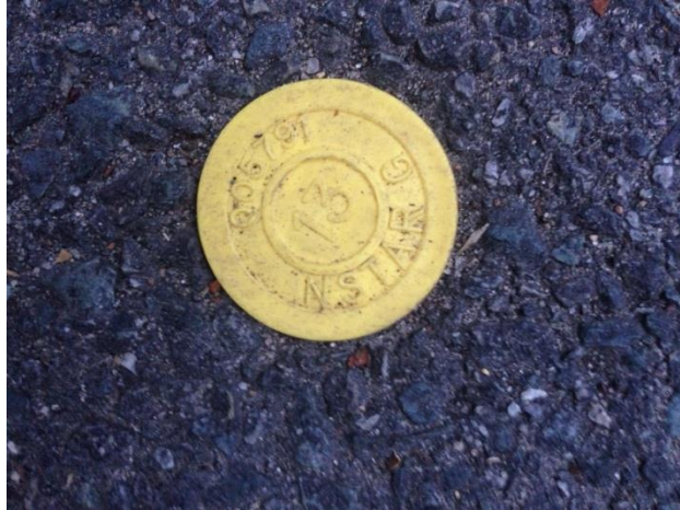
Figure 18. A Plastic tracking tag used by Eversource (formerly NSTAR)
