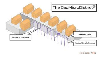
management while reducing total energy load needed through load sharing and load cancelling. GeoMicroDistricts interconnect like Lego® blocks, building thermal energy grids that combine the efficiency of utility-scale load with the ability to island.
