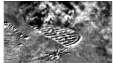
Thermal imaging of gas emitting from a sewer
