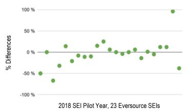
The leak extent measurement at individual leaks remained relatively consistent, over an average of four months, even when the same leak was measured by different personnel from two different organizations. This method appears to be robust.
