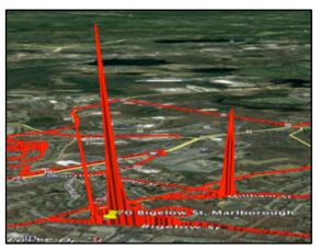
A known leak aligns with CRDS mobile survey data
