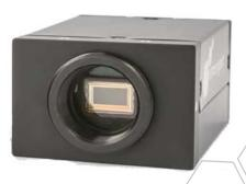
The HT Series cameras are our newest product family with camera options of 2MP, 4MP, 12MP, or 20MP. These cameras are smaller in physical size and come equipped with CAT6A 10GBaseT Connections. They have the more familiar ethernet connection similar to GigE but 10x the speed. Cable lengths can go up to 100M.
