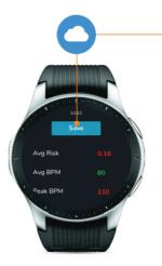
3 Data is continuously collected on the watch and uploaded to the cloud when connectivity is established via wifi or cellular.
