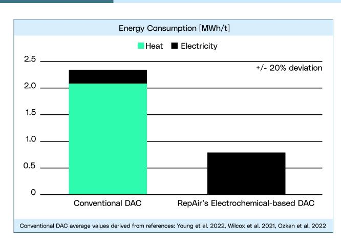
The core units exhibit low energy consumption of less than 0.6 MWh per ton CO<sub>2</sub>, including regeneration, resulting in a total energy consumption of less than 1 MWh/tCO<sub>2</sub>. Moreover, the carbon footprint is below 5% - less than 50kg of CO<sub>2</sub> are emitted for every ton of CO<sub>2</sub> removed. The system is estimated to have a compact footprint of ~15 tCO<sub>2</sub>/m<sup>3</sup>, further highlighting its efficiency and scalability.
