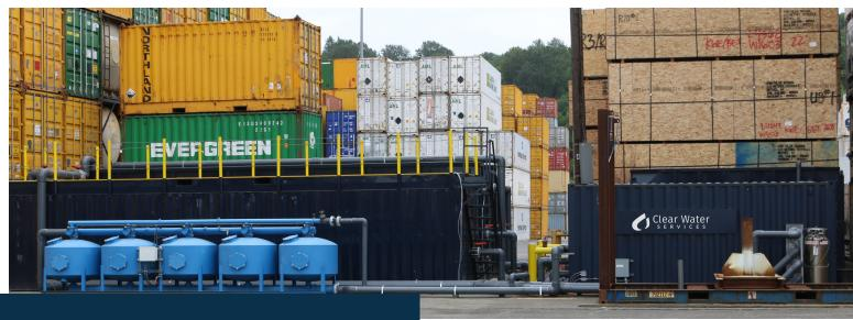
The CS-20 is a patented mobile unit designed to treat sediment-laden stormwater, groundwater, and industrial wastewater.
