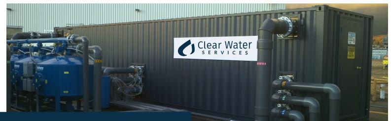
The CS-40 is a patented mobile unit designed to treat sediment-laden stormwater, groundwater, and industrial wastewater.
